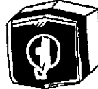
D.P. Switch (Dyna King) Flush D.P. Dyna King with Fuse Carrier
